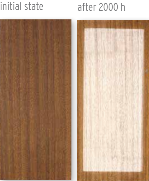
Teak completely bleached surface, major structural differences early wood / late wood
