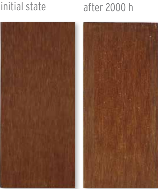
Resysta + Stain (Walnut) very slight change in color, individual white particles slightly visible
