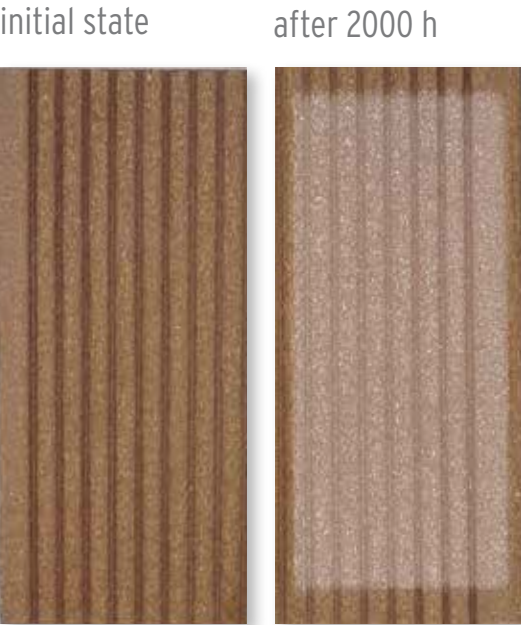
WPC very severe change in color (bleaching), several white particles individually visible
